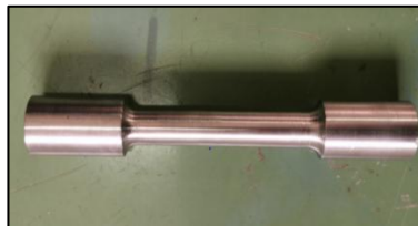
Fig.3.1 samples where machining on a lathe machine
