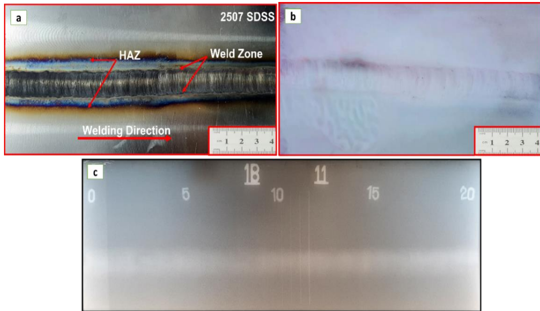
Fig. 7 (a)Top view of 2507 SDSS with multi pass GTAW, (b) image for liquid penetration test of 2507 SDSS with multi pass GTAW, (c) Radiographic images of the 2507 with multi pass GTAW.
