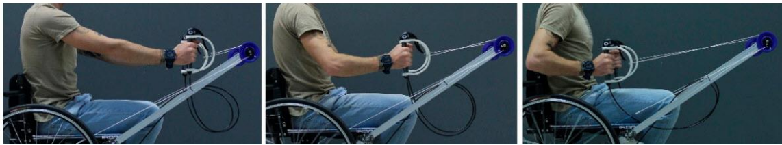
Figure 6: Innovative system of propulsion for MWs [24].
