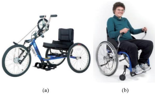
Figure 4: Some types of MWs: (a) Crank-propelled wheelchairs, (b) Lever-propelled wheelchairs [15].
