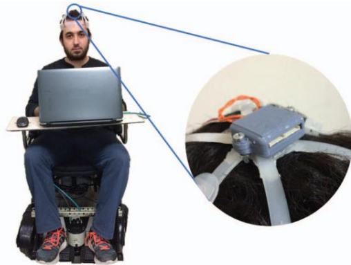
Figure 26: IMU with a head gesture for controlling wheelchairs [103].
