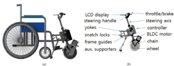
Figure 8: Easy-docking mechanism: (a) 3D design of the mechanism, (b) Parts of the wheelchair driving module [14].
